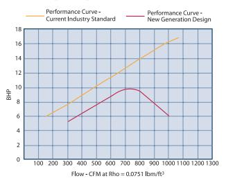
Figure 4 – Motor Power Comparison, units are matched in flow/pressure performance; new-generation product is matched to current industry standard performance curve via turn-down.
