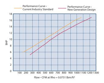
Figure 3 – Motor Power Comparison, units at constant 18,000 RPM impeller speed. Even though blower speed is the same, this comparison is misleading because pressure delivery, i.e., performance is not equivalent, as was shown in Figure 1.
