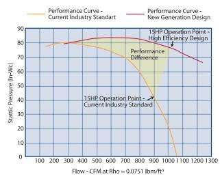
Figure 1: Direct Performance Comparison, units at constant 18,000 RPM impeller speed, with 15HP operating point defined for both. New-generation unit also delivers far greater performance for the same 15HP energy cost.
